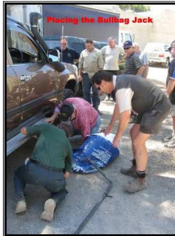
The exhaust jack was demonstrated and then applied to various vehicles to test suitability. Although not as bullet proof as the Hilift the Bullbag has an advantage in ease of stowage and good adaptability to many standard vehicles. Brian was impressed by the lift we did on his Triton. Thanks go to Ray in demonstrating smoke and soot hazard when operating the exhaust jack!
