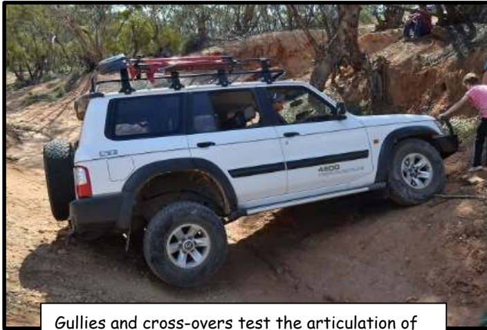
Gullies and cross-overs test the articulation of the Patrol - note the front left wheel dug in to the top of the rim in the moist soil.
